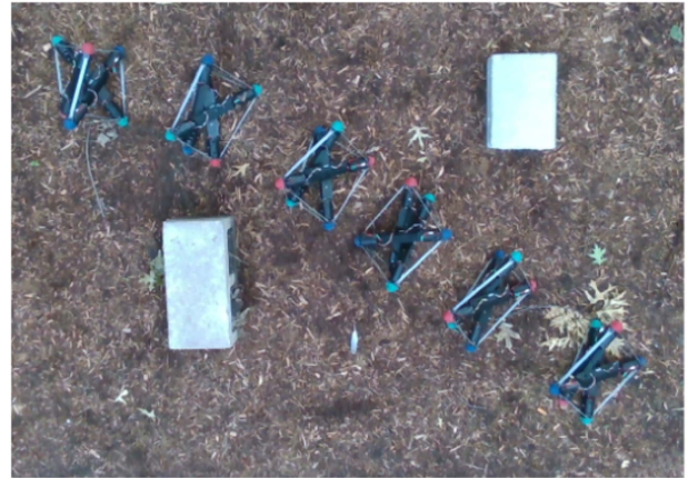
Fig. 1. The open-source tensegrity robot moving around obstacles outdoors starts from the top left and autonomously navigates to the bottom right.
